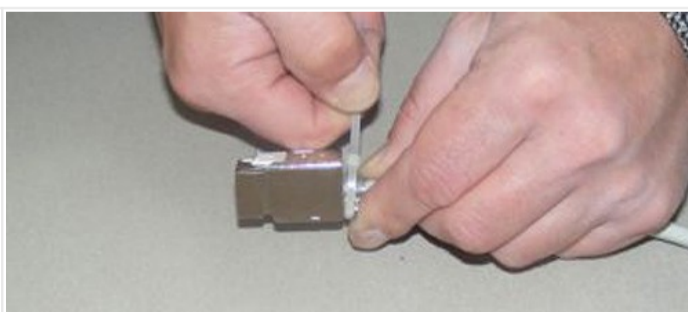
Move the shielded braid back (twisting at the same time) so that it sits under the rear tag, then apply the supplied cable ties to secure it to the body
