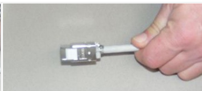
The finished connector should not show any stray wires. The jacket should reach to the rear of the connector. The braid should be tidy beneath the tag
