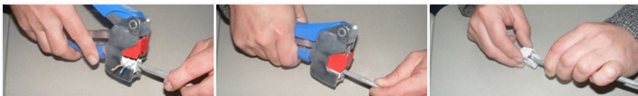
Insert jack into ezi-TOOL with red cutting blade
