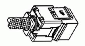
Step 4: Press tool to terminate the jack and cut off the excess wires
