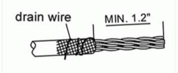
Step 1: Strip off at least 1.2 inch of jacket from end of cable. Wrap the drain wire around the cable
