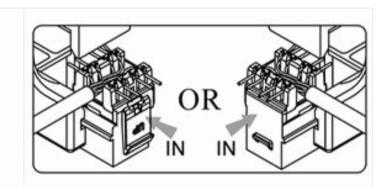
Step 3: Insert the jack into the tool guides with the cable coming out to the side
