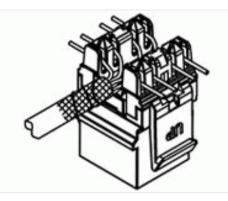
Step 2: Press the wires through the projecting portion of terminals until fixed (T568A/T568B)
