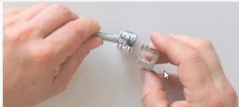
Check terminations, then place top cap onto jack with the slot facing the wire, and click into place
