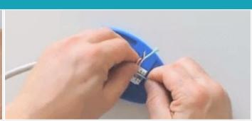
With twists right up to the IDC terminals, load the jack terminals with the wires in the correct color order
