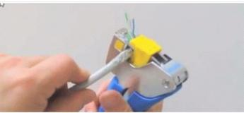
Squeeze handles together terminating and trimming wires
