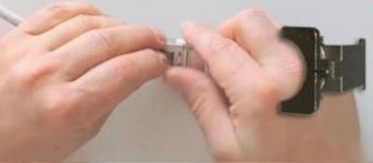
Take the other half of the shield clamp and insert into main body, then push down until it clicks into place
