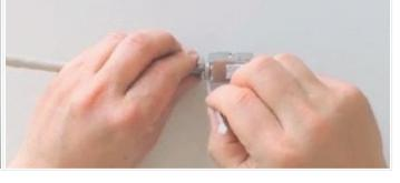
Finally, take the supplied cable tie and secure the two halves of the clap together
