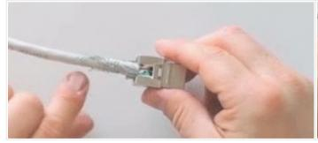
Move the cable into a straight up and down direction, and then tidily push braid up and under the shielded tag at the back, twisting the braid as you push it up
