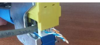
Squeeze handles together terminating and trimming wires
