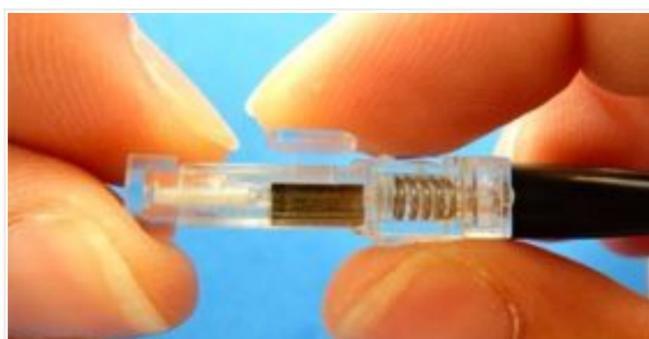
How to re-use connector : Insert the connector insert release key; press down to release the metal button
