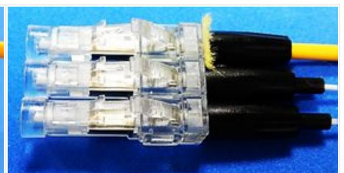
To make as duplex, triplex & quadruplex : clamp connectors side by side to create multi configurations
