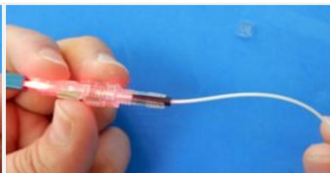
Form a small curve. Then, press metal button to connect fibers. You will see no leakage of red light for a low loss
