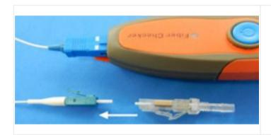
Remove dust cap and clean ferrule. Connect QLC with fiber VFL to verify connections
