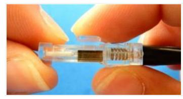
How to re-use connector: Insert the connector insert release key; press down to release the metal button
