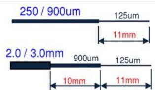
Slide on correct boot, and screw cover. Prepare fiber as below. Strip and clean it. Cleave fiber precisely
