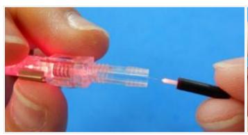
Insert fiber to LC connector until it touches the fiber inside
