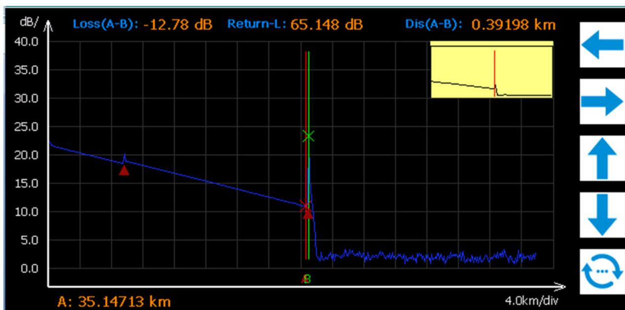
Fig.3-10 Return loss measurement
