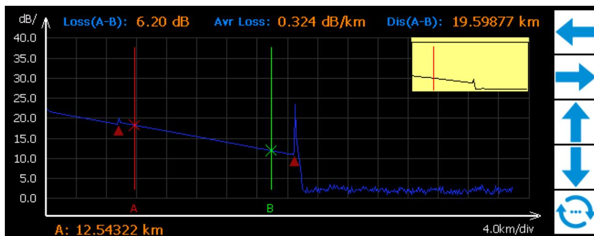
Fig.3-8 Average Loss Measurement
