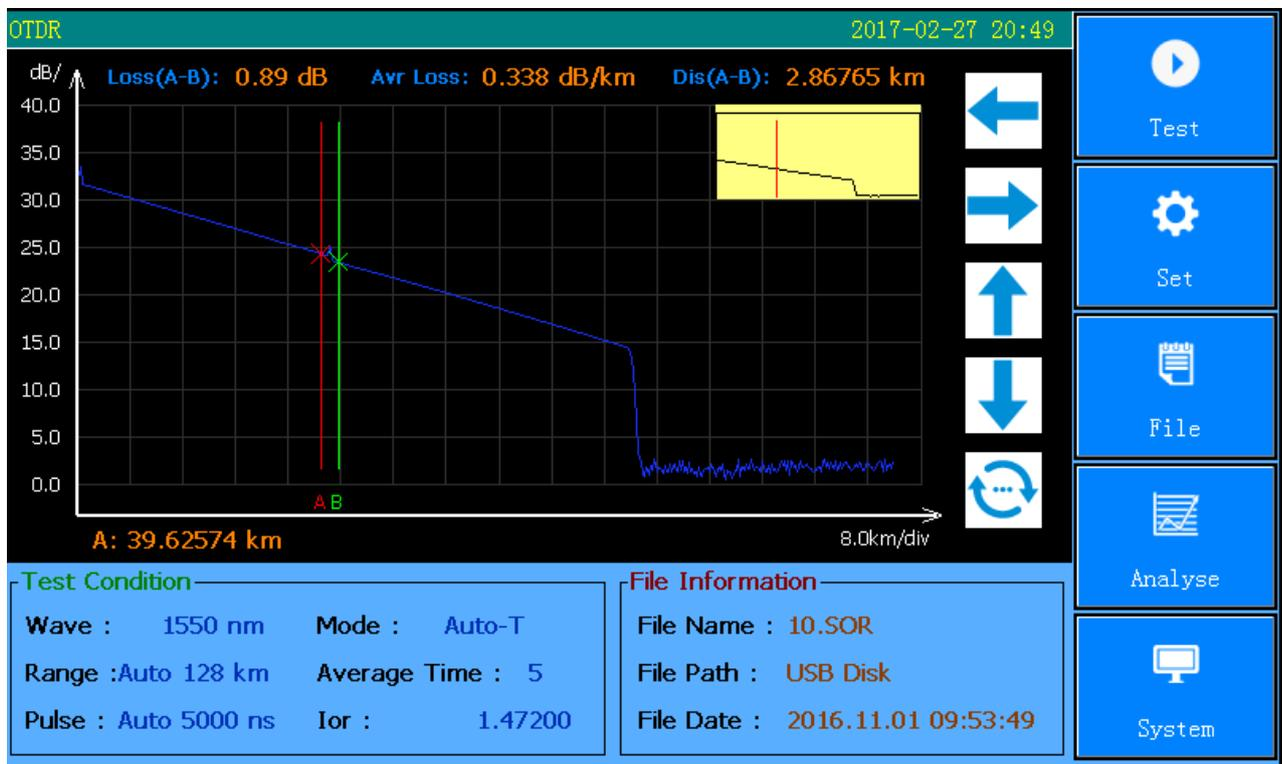
Fig.3-5 Connection Loss Test
