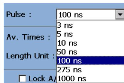
**Test mode: Mode for selecting OTDR scan type.**
