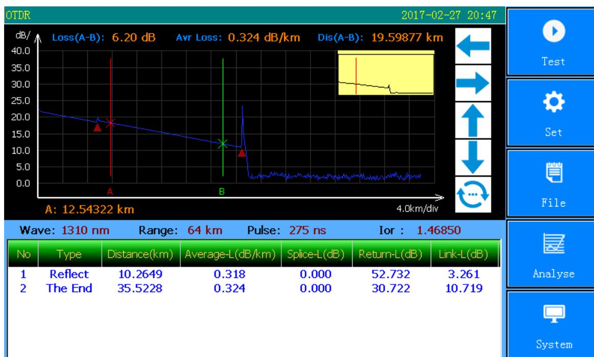
Fig.3-4 Average Loss Test
