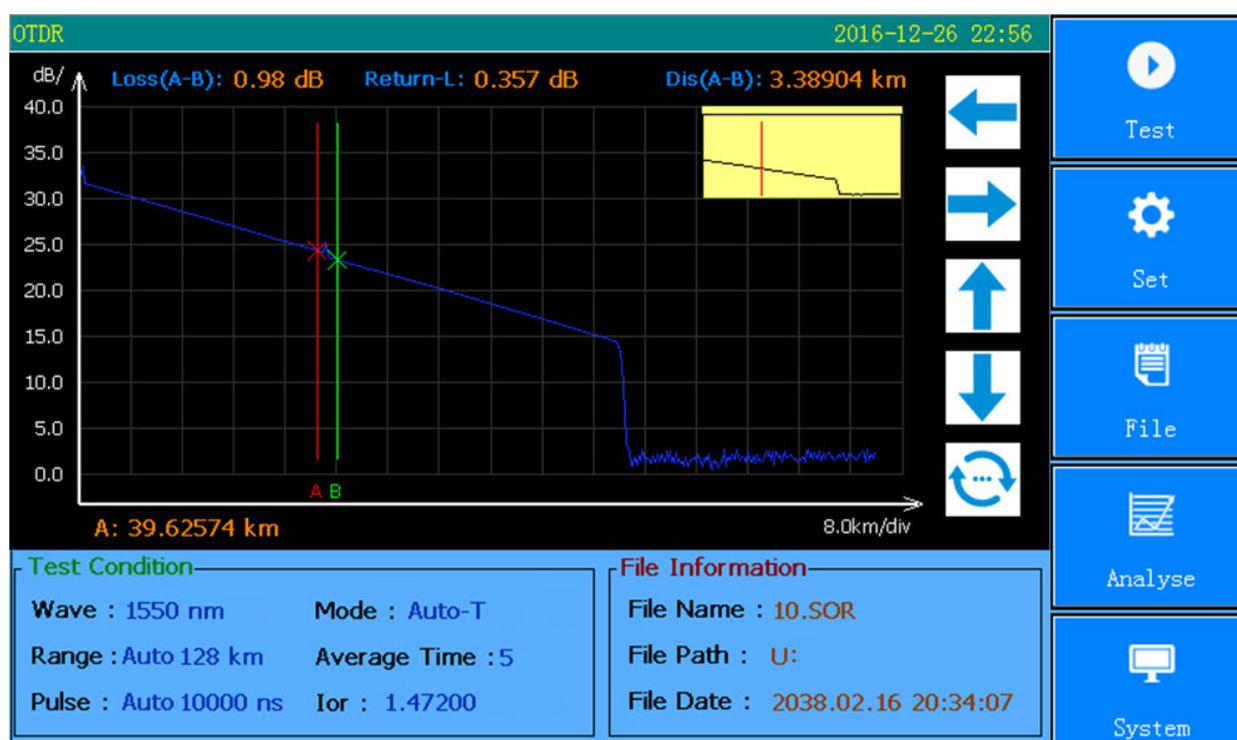
Fig.3-9 Connection Loss Measurement
