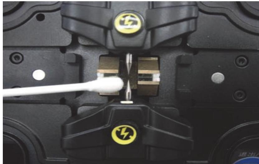
Figure 3-2 Clean the Electrodes
