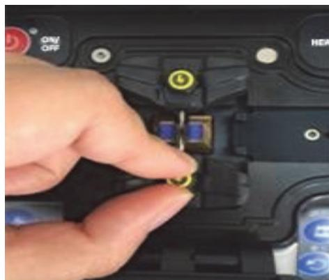
Figure 3-3 Electrodes - replace
