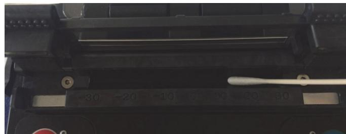
Figure 3-7 Clean the Heating Plate
