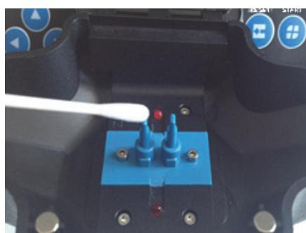
Figure 3-6 Clean the Fiber Presser Foot
