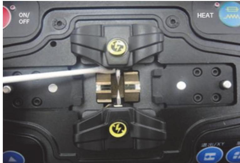
Figure 3-5 Clean the Microscope
